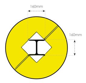
Height: 1m Diameter 600mm Weight: 23kg Wall Thickness: 6.4mm 210mm
